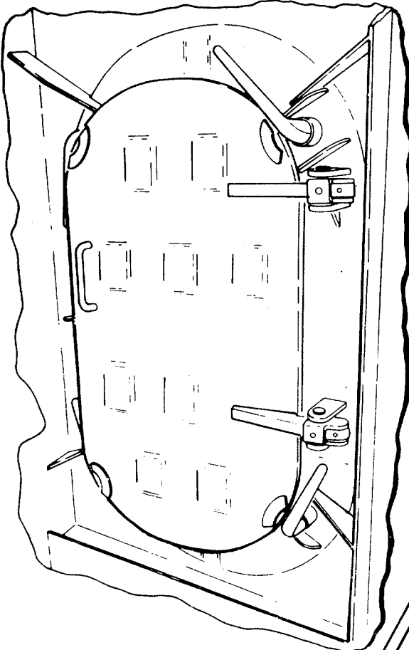
WATERTIGHT DOOR (TYPICAL)
